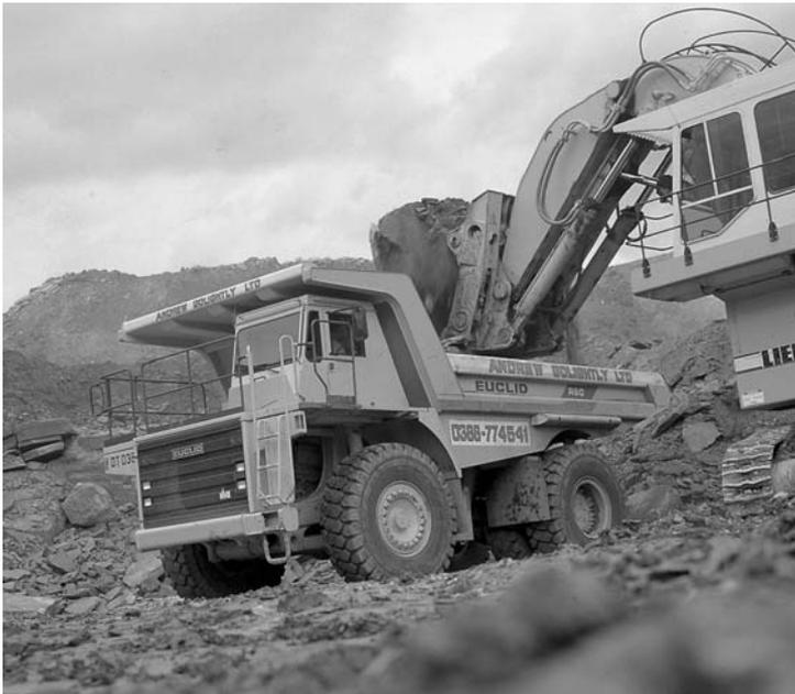
**Plate 2b.** A Euclid R60 522 kW dump truck, 36 m<sup>3</sup> heaped capacity. VME Construction Equipment GB Ltd, Duxford, Cambridge, UK
