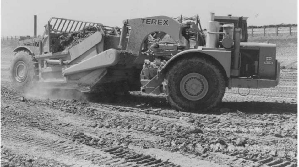
**Plate 3a.** A Terex TS24C 552 kW twin-engined 36 m<sup>3</sup> capacity scraper for earth-moving. Terex Equipment Ltd, Motherwell, Scotland
