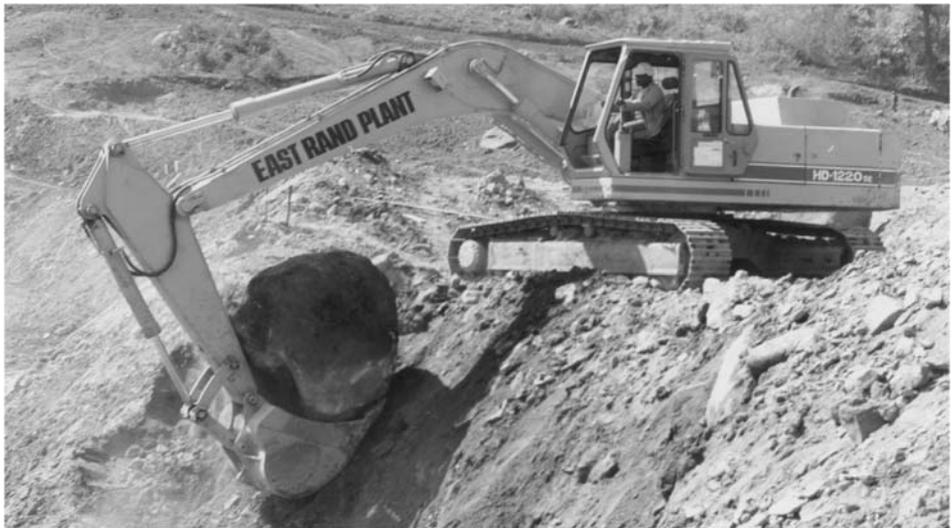
**Plate 3b.** A Kato 162 kW tracked excavator, with 1.6 m<sup>3</sup> bucket. ACP Holdings, Leicester, UK
